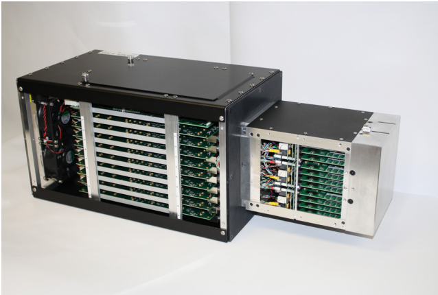
Fig. 1. Showing a complete Anger Camera Assembly. The “snout” on the right contains the optics package and preamp electronics. The signal processing boards are also visible within the body of the detector.
