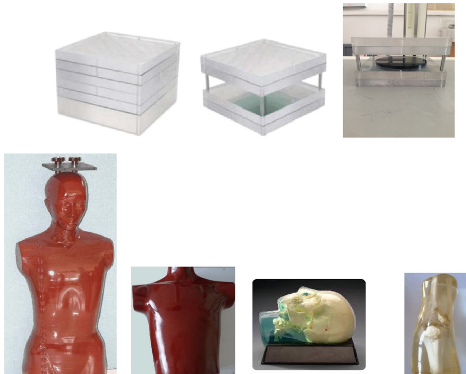
Fig. 1. Top: PMMA slab (left), ANSI chest phantom (middle) and ANSI chest with contrast test tool (right). Bottom: anthropomorphic phantoms; Rando phantom, thorax phantom, skull phantom and extremity phantom (left to right).
