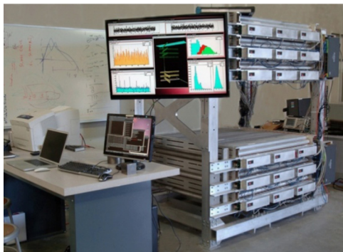
Fig. 1. Photograph of the mini muon tracker (MMT). The MMT consists of an upper and a lower tracker. Each tracker has 12 planes of drift tube detectors, the detector orientations were crossed between planes to provide tracking in both horizontal directions. Objects for study were placed in the approximate two-foot (60 cm) gap between the two detector “supermodules”.
