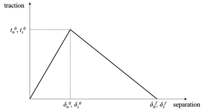
Fig. 2. Traction-separation law with linear softening.
