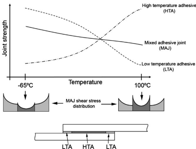
Fig. 1. Working principle of the mixed adhesive joint concept.
