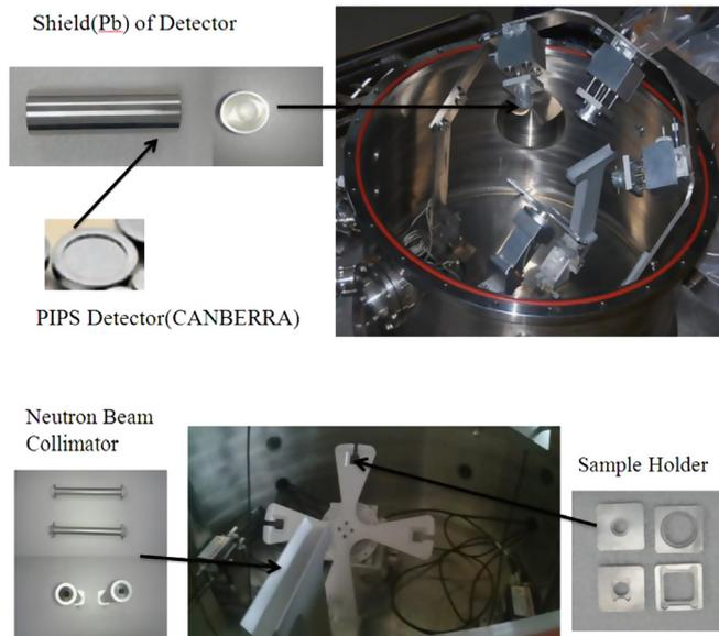
Fig. 2. Inside of the target chamber.
