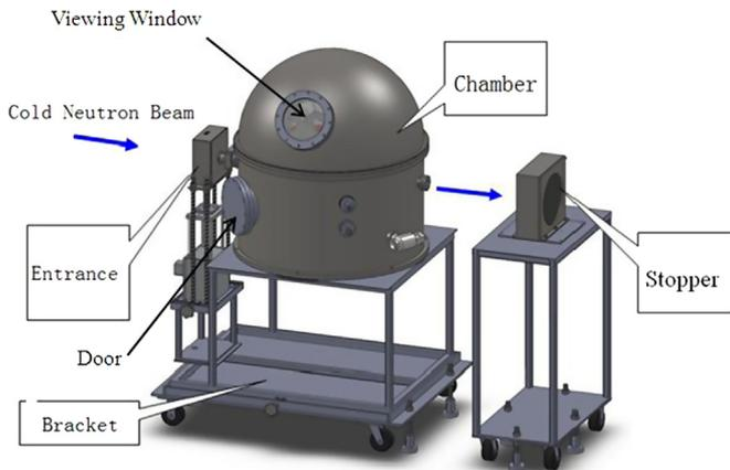
Fig. 1. Layout of the INPC-NDP structure.
