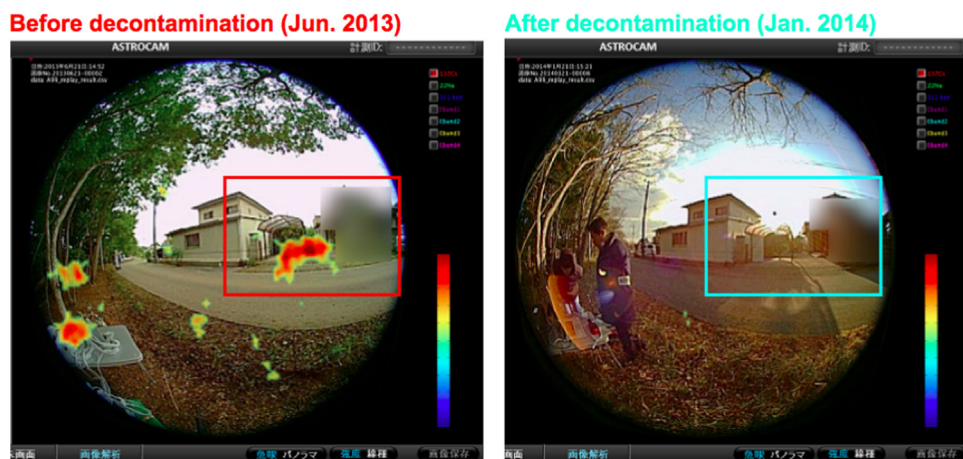
Fig. 2. One example demonstration in the 20 km zone of the nuclear plant. ASTROCAM was located at the same position, both (left) before radioactive clean-up in June 2013, and (right) after radioactive clean-up in January 2014.
