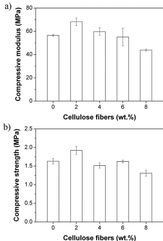
Fig. 1. Compressive mechanical properties for PF and CRPFs with 2, 4, 6 and 8 wt.% of cellulose fibers: a) Modulus (MPa) and b) Strength (MPa).
