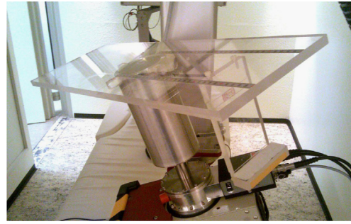
Fig. 2. Detector with the PMMA plate mounted on top and the source holder hanging from the PMMA plate. The holder has an additional white part not relevant for the purpose of this work.
