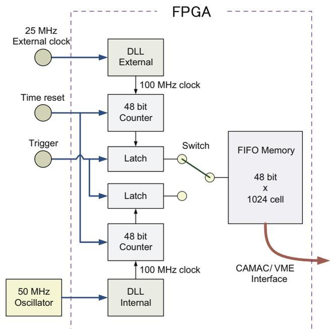
Fig. 2. Block diagram of time-stamp circuit implemented in FPGA.
