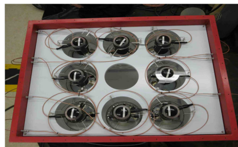
Fig. 1. A schematic (left) of the detector showing a cut away of the 73 cm deep source deployment well/cavity and PMT placement (PMTs not shown). To the right is the finished detector immediately after PMT placement inside and prior to the installation of the lid and well.
