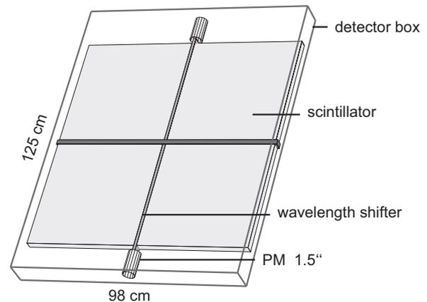
Fig. 2. Schematic view of a scintillation detector. Sheets of plastic scintillator are read out by photomultiplier tubes via wavelength shifter bars [14].
