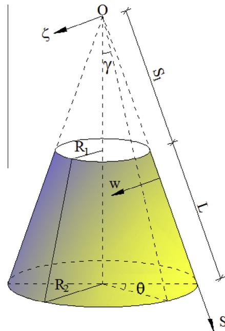
Fig. 1. The schematic configuration of an FGM conical shell and coordinate system.
