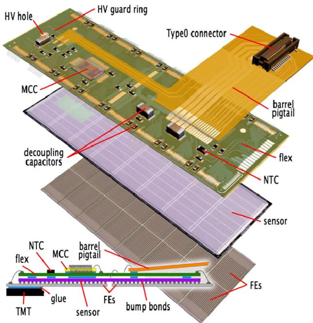
Fig. 2. Exploded Pixel Detector module, showing the 16 Front-Ends, sensor tile and flex PCB with connector.
