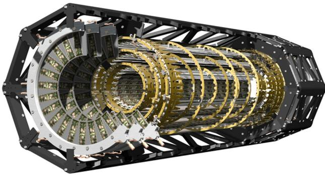
Fig. 1. Computer generated picture of the partially opened Pixel Detector in its carbon support structure.
