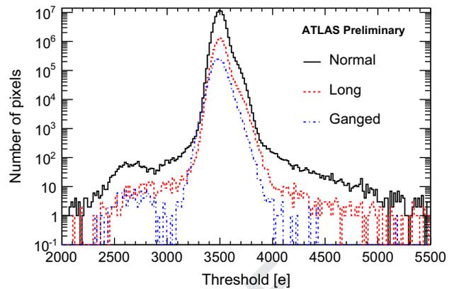
Fig. 3. The calibrated per pixel threshold. Overlaid are the different pixel sizes [3].
