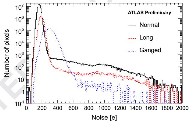
Fig. 4. Measured noise per pixel. Overlaid are the different pixel sizes [3].
