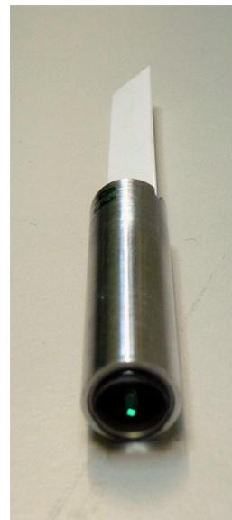
Fig. 3. A detection unit ready to be connected to a SiPM.
