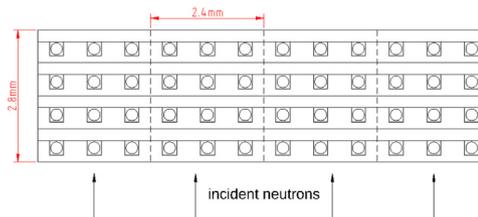
Fig. 4. Cross-sectional view of a possible multi-channel detector repeating laterally and vertically the pattern of the single channel detection unit with three fibers. The channels are delimited by the dashed lines. Each channel contains 12 WLS fibers.
