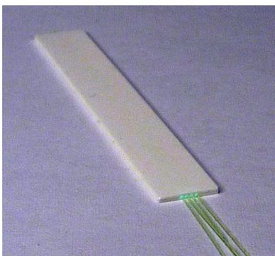
Fig. 2. The 4-fiber detection unit before assembling with a fiber holder.
