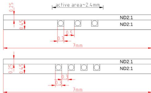
Fig. 1. Cross-section of the detection units with three fibers (top) and four fibers (bottom).
