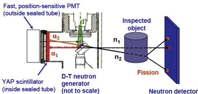
**Fig. 1.** In tagged neutron interrogation, the associated particle detector detects the alphas from the DT reaction within the DT neutron generator. The neutron associated with the detected alpha particle passes through or interacts with the inspected object. The neutron or its interaction product(s) may be detected in the neutron detector [1].
