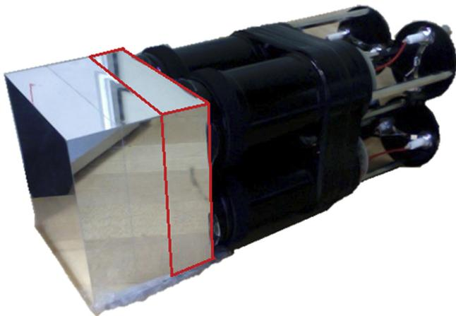
**Fig. 2.** The block detector based upon Oak Ridge National Laboratory design for APNIS. The red boxes outline the segmented light guide. Located to the left of the light guide is the  $10 \times 10$  EJ-200 array. Located to the right of the light guide is the  $2 \times 2$  array of PMTs. (For interpretation of the references to color in this figure caption, the reader is referred to the web version of this article.)
