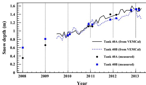
**Fig. 2.** Accumulation of snow over time, for the two tanks of one IceTop station [9]. Direct measurements of snow depth are shown with solid symbols. Indirect measurements using calibration curves (VEMCal data) are shown with lines.
