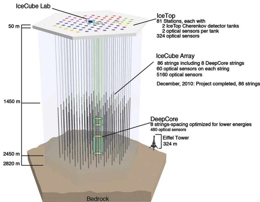
**Fig. 1.** Sketch of the IceCube Observatory. IceCube in its 2006–2007 configuration is shown in red and referred to as IT26/IC22 (26 IceTop stations/22 in-ice cables). Other configurations are IT40/IC40 (2007–2008) in green, IT59/IC59 (2008–2009) in purple, IT73/IC79 (2009–2010) in blue, and IT81/IC86 (2010–2011 and subsequent seasons) in yellow. (For interpretation of the references to color in this figure caption, the reader is referred to the web version of this paper.)
