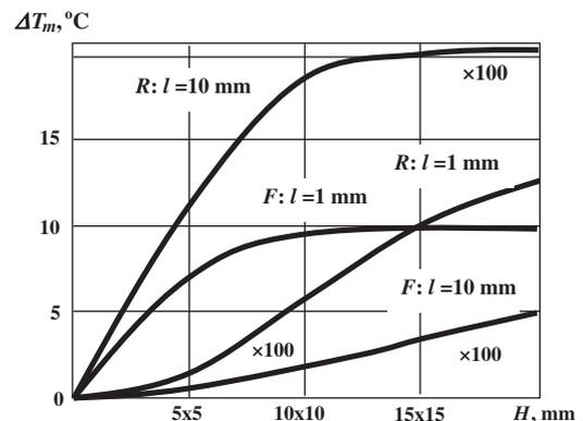
Fig. 2. Differential temperature signal vs. defect size in the inspection of a 11.6 mm-thick CFRP sample (see the legend in Appendix,  $d = 0.1$  mm).
