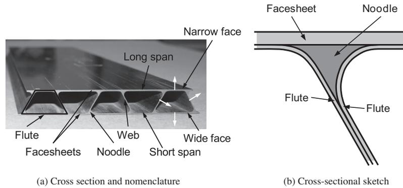
Fig. 1. Cross section of an unjointed fluted-core composite panel.
