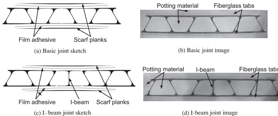
Fig. 2. Joint configurations. The grey lines in (a) and (c) represent film adhesive.
