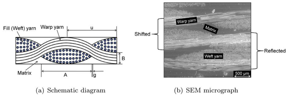
Fig. 1. Cross-section of the plain-weave fabric glass/epoxy composite. (a) Schematic diagram. (b) SEM micrograph.
