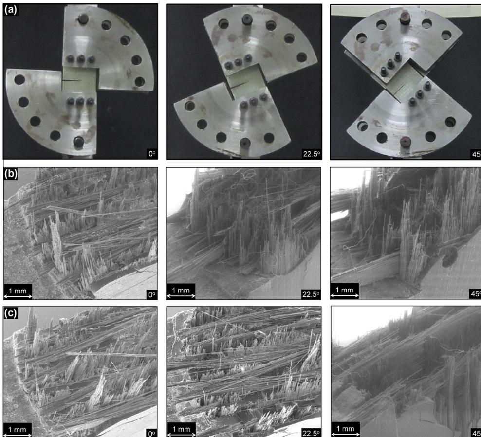
Fig. 2. (a) Experimental loading arrangement for different loading angles. (b) SEM images of fractured surface of the upper half of the specimen. (c) SEM images of fractured surface of the lower half of the specimen.
