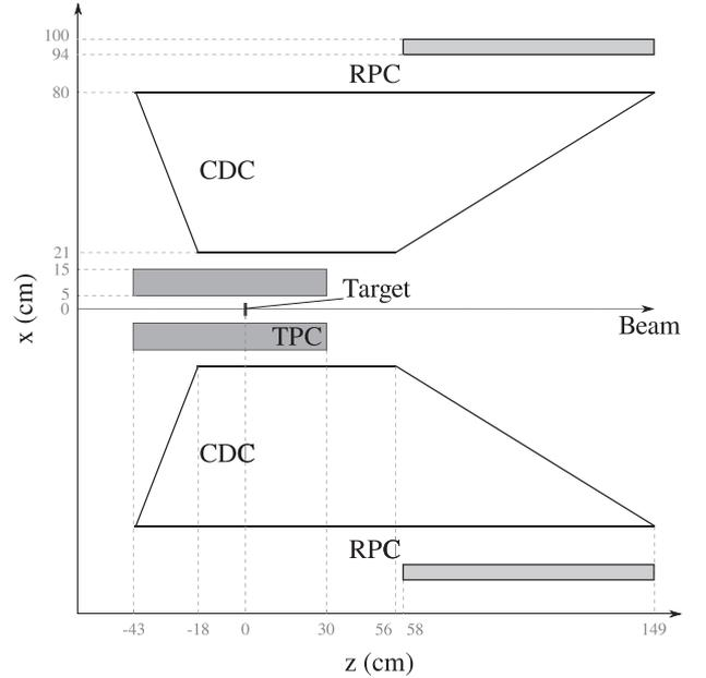
**Fig. 2.** Cross-section of the GEM-TPC + FOPI setup. Only the detectors relevant for this analysis are shown. The given dimensions are rounded values.
