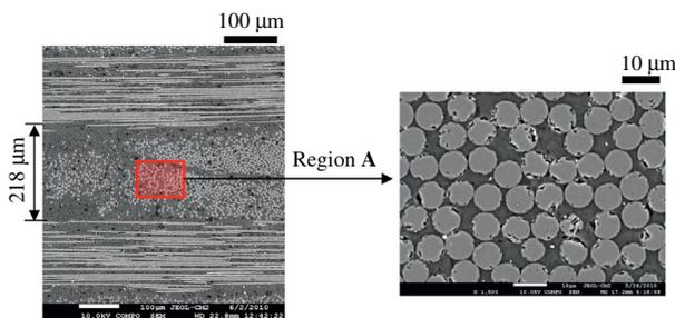
Fig. 1. Fibre arrangement as observed from a scanning electron microscope.
