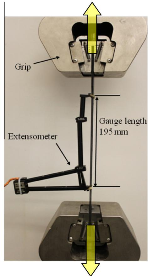
Fig. 2. Tensile test setup.
