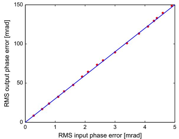
Fig. 1. The output phase error dependence on the seed laser phase error for the case of 1 modulator period, the slope of the blue line is 30, the red dots are the simulation results. (For interpretation of the references to color in this figure legend, the reader is referred to the web version of this article.)
