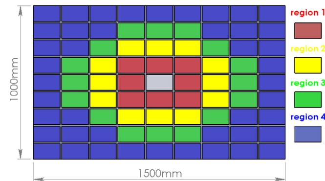
Fig. 1. Particle rate distribution in the full area of CBM-TOF.
