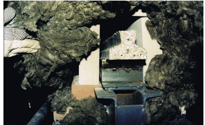
Fig. 4. First series: positioning of the beam in the oven.
