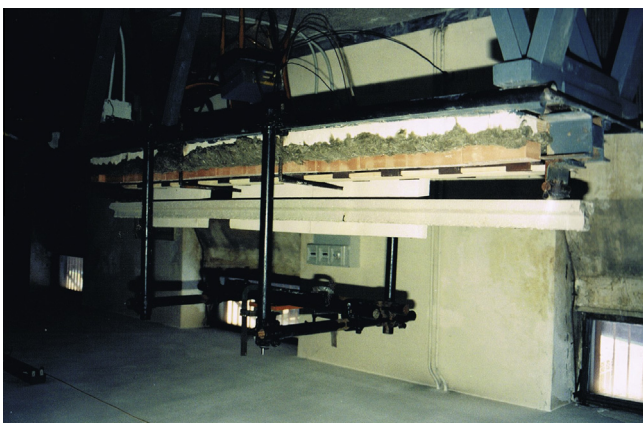
Fig. 3. First series: the pre-compressed beam and the supporting structure.
