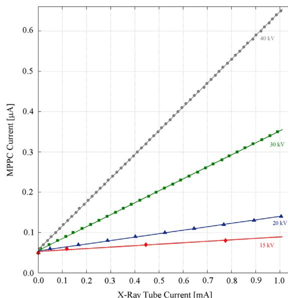
Fig. 2. MPPC current as a function of X-ray tube current for different accelerating voltages.
