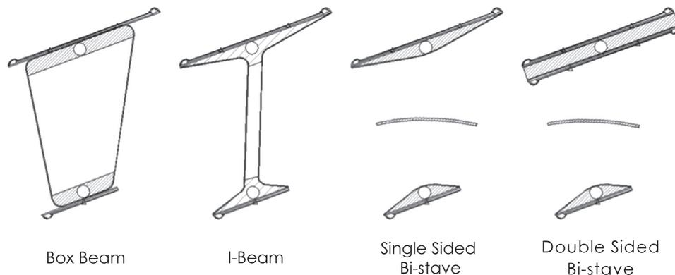
Fig. 2. Comparison of four different approaches to supporting two detecting layers.
