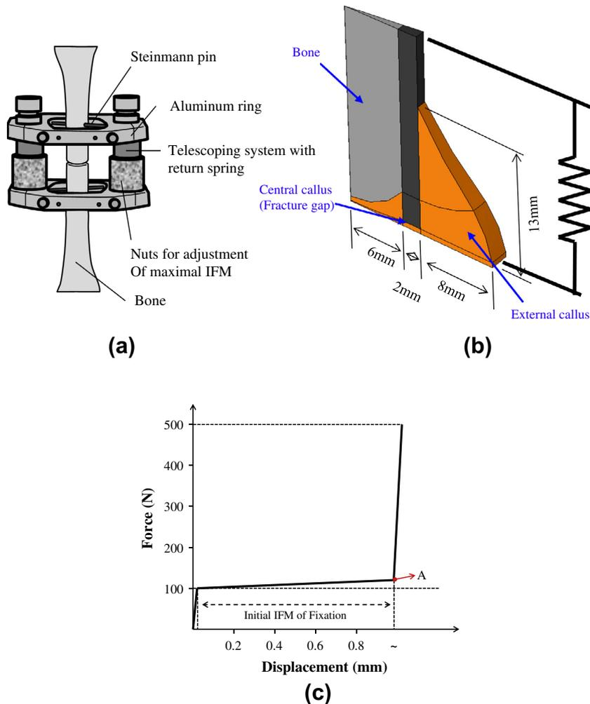
Fig. 1. A fractured sheep tibia with an external fixator; (a) schematic drawing, (b) finite element model, (c) a piece wise spring constant of an external fixator.
