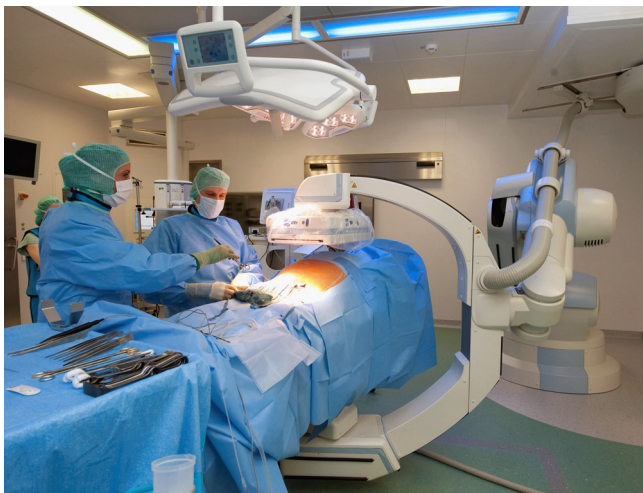
Fig. 1. Robotic C-arm system used in a hybrid operating room for endovascular aortic repair including coiling of the arteria mesenterica inferior. Courtesy of Dr. Johannes Gahlen, Hospital Ludwigsburg, Germany.
