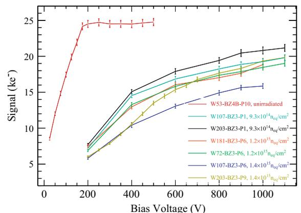
**Fig. 2.** Most probable charge after pion irradiation doses. The result for an unirradiated device is shown as a reference.
