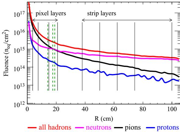
**Fig. 1.** Equivalent fluence for different hadron types in dependence of the distance from the interaction point for an integrated luminosity of  $3000 \text{ fb}^{-1}$ . The data is shown for  $z=0$ , a safety factor of two was applied, data from Ref. [2]. The dashed lines indicate the radii corresponding to the irradiated fluences.
