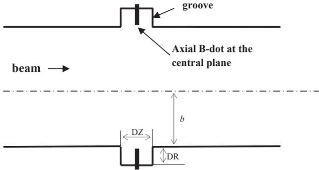
Fig. 2. Groove for practical axial B-dot.
