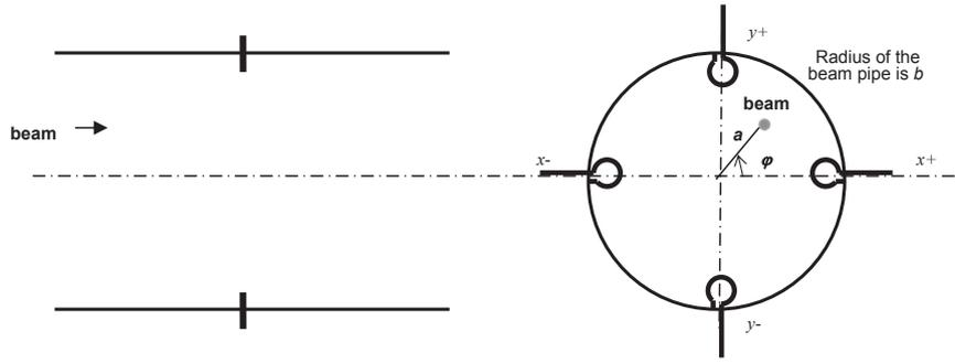
Fig. 1. Arrangement of axial B-dot measuring beam tilt [7].
