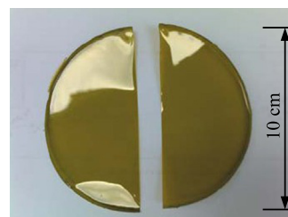
Fig. 2. Photograph of a D-polystyrene foil. The foil thickness increases from 70 \mu\text{m} in the center to 100 \mu\text{m} at the edge.
