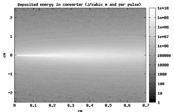
**Fig. 3.** FLUKA simulation of energy density deposited per pulse ( $7 \times 10^{12}$  electrons).
