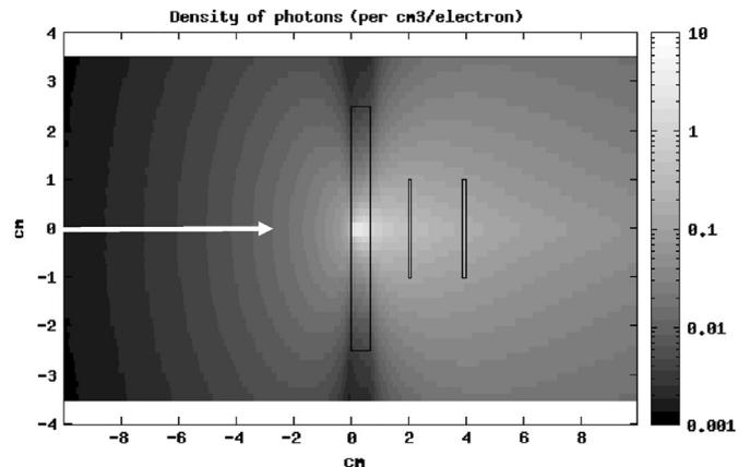
**Fig. 2.** FLUKA simulation (with 1 keV lowest transport limit for photons and electrons) of bremsstrahlung production of photons in 0.7 cm thick, 7 cm diameter tungsten target by 0.5 cm diameter pin electron beam (35 MeV).
