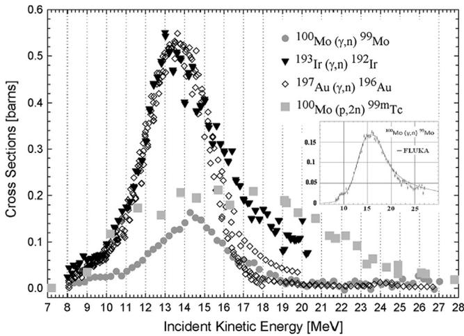
**Fig. 1.** Cross sections for  $^{100}\text{Mo}(\gamma, n)$  [7],  $(p, 2n)$  [5,6] and  $^{193}\text{Ir}(\gamma, n)$  [8]  $^{197}\text{Au}(\gamma, n)$  [9] reactions versus incident beam energy. Data are taken from <http://www.nndc.bnl.gov>. In the inset solid line represent used in FLUKA code the respective cross sections for  $^{100}\text{Mo}(\gamma, n)$ .
