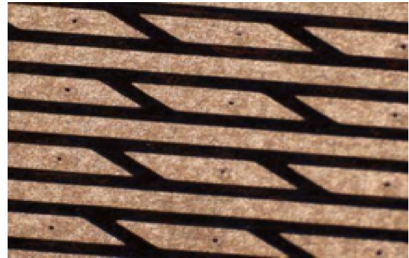
Fig. 3. The X-V patterned read-out plane with straight longitudinal X strips interleaved by parallelogram-shaped pads connected through vias to form V strips at \sim 25^\circ .
