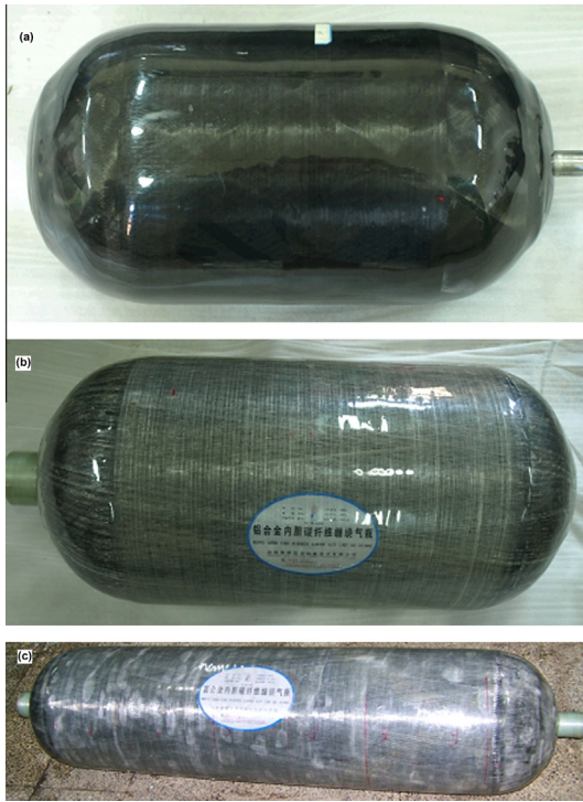
Fig. 1. (a) 15 L composite vessel-A, (b) 74 L composite vessel-B and (c) 150 L composite vessel-C.
