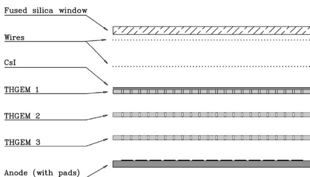
Fig. 1. Scheme of a THGEM-based photon detector.
