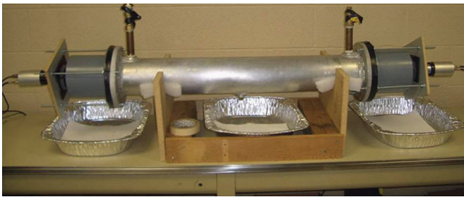
Fig. 1. The setup of our liquid scintillation detector. The aluminum foil pans are required for safety in case of leaks.
