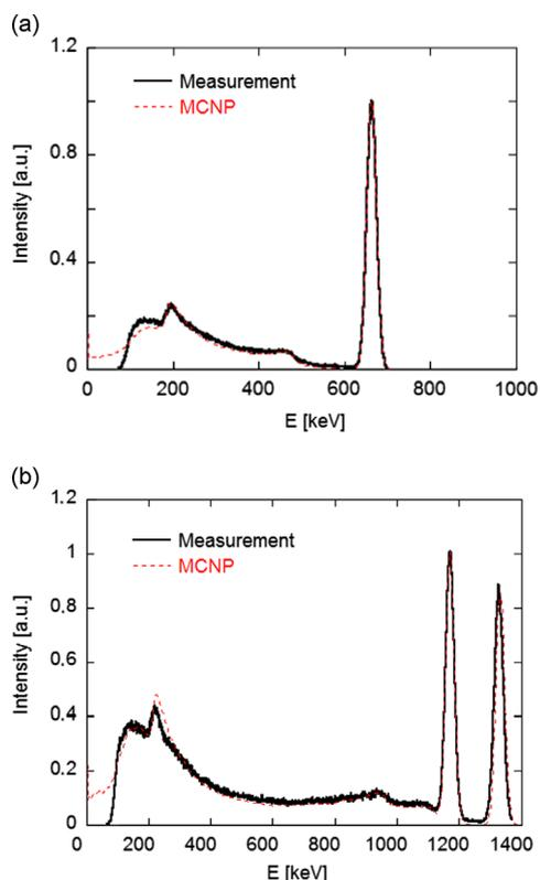
Fig. 1. Simulated and measured energy spectrum using a LaBr<sub>3</sub> scintillator for a <sup>137</sup>Cs (a) and a <sup>60</sup>Co (b) radioactive source.
