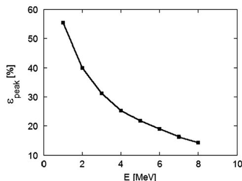
Fig. 2. Simulated full-energy-peak efficiency as a function of the  $\gamma$ -ray energy for a 3 in. × 6 in. LaBr<sub>3</sub> scintillator.
