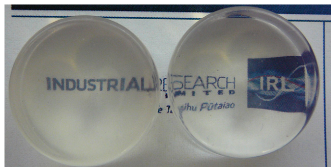
Fig. 1. Photo of scintillator samples, 1.25 wt% enriched LiME (left) and 10 wt% enriched LiME (right).
