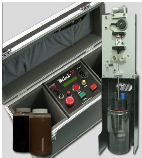
Fig. 1. A photograph of portable nano-colloid synthesizer (NTi-MiniP).
