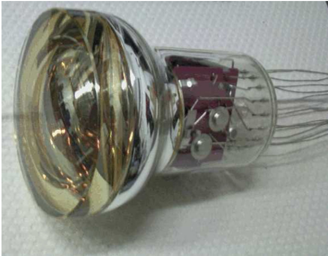
Fig. 1. The new Hamamatsu R6233mod PMT.
