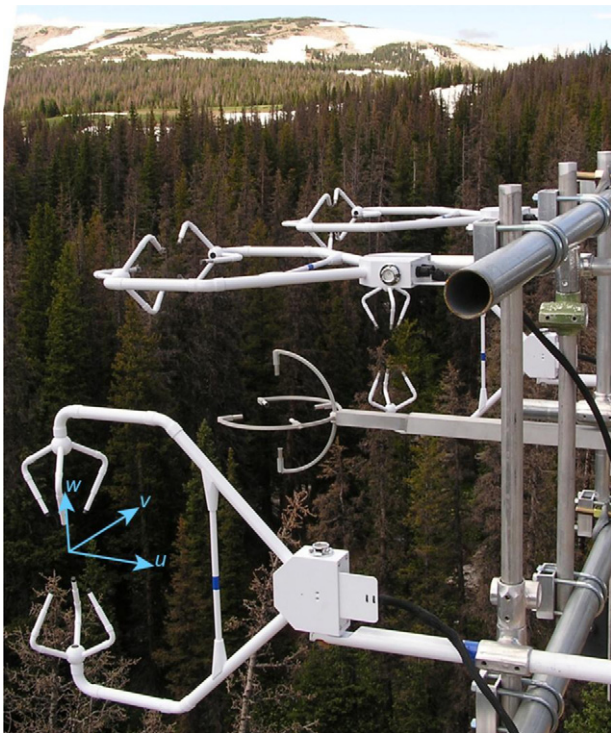
Fig. 1. Photograph of the experimental setup. Position 1 is in the bottom left. The CSAT3 sonic anemometers in positions 2 and 4 are mounted in the horizontal orientation. The u , v , and w axes are shown in light blue for position 1. (For interpretation of the references to colour in this figure legend, the reader is referred to the web version of this article.)
