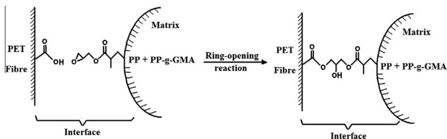
Fig. 1. Schematic representation of reaction between PET end-groups and GMA moieties grafted onto PP backbone.
