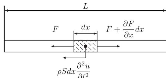
Fig. 1. Forces acting on an infinitesimal beam segment subjected to longitudinal natural vibration.
