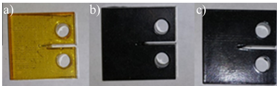
Fig. 2. CT samples after curing process (a) baseline, (b) 0.1 wt% and (c) 0.5 wt% NGP.
