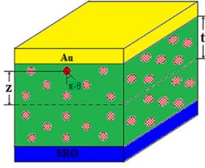
**Fig. 1.** (Color online.) The illustration to granule/matrix composite structure with Ni/PZT component.
