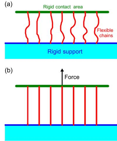
Fig. 1. Scheme illustrating two flat rigid contact areas, linked by flexible elastic chains, (a) without and (b) with the external force.
