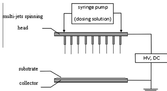
Fig. 1. Schematic diagram of the multijet electrospinning apparatus.
