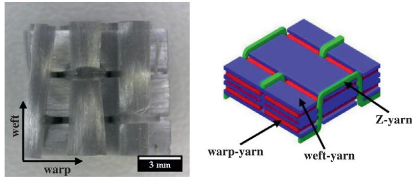
Fig. 1. Architecture of the tows inside the non-crimp 3D orthogonal weave preform [11]: photo (left) and schematics (right) of the unit cell.
