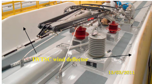
Fig. 2. Application of IWTSW in wind deflector of CRH trains.
