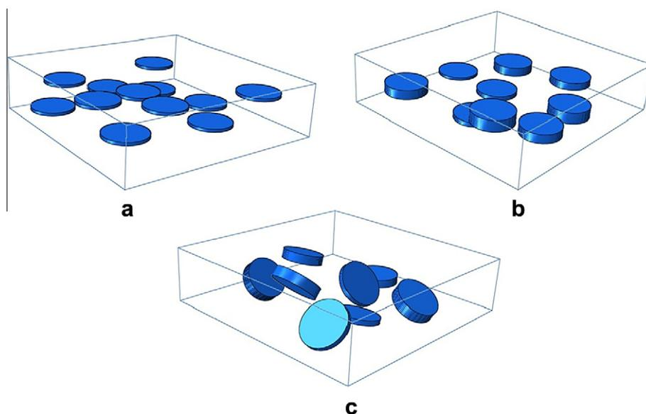
Fig. 1. Examples of 3D models of nanocomposites with different arrangements of nanoplatelets. (a) Unit cell with aligned horizontal exfoliated nanoplatelets. (b) Unit cell with aligned multi-clusters. (c) Unit cell with randomly oriented clusters.
